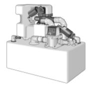
*Fully Integrated Design.* Dometic HTS-EC systems combine the vacuum generator, level indicators, discharge pump and holding tank into one, easy-to-install package. Available in 35-, 60-, and 90-liter capacities.
